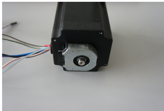
Fig. 3.11: Motor with attached encoder
