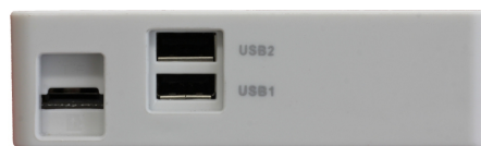
Fig. 7.3: View from the right. Left to right: micro-SD card connector, two USB type A female connectors
