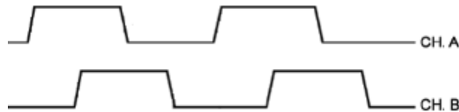
Fig. 4.17: The signals at CH A and CH B outputs of quadrature encoder
